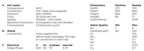
Refer operator manual for installation instructions. Isolating switch must be within 1m of, and not directly behind the machine. Isolating water valve must be readily accessible. \*Consumption may vary with site conditions.
