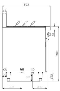
Gas Inlet 1/2" BSP Female Drain Outlet 1-1/4" BSP Male
