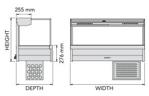
Note: For overall height dimensions, add height of motor cage (450 mm).
